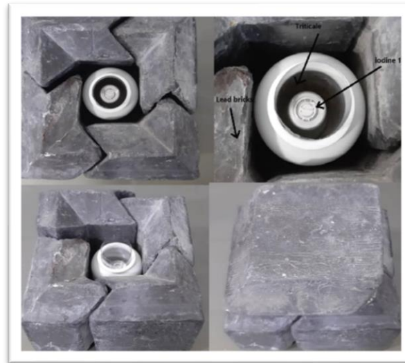
Figure 1. Placement of seeds for radiation with lead shield
